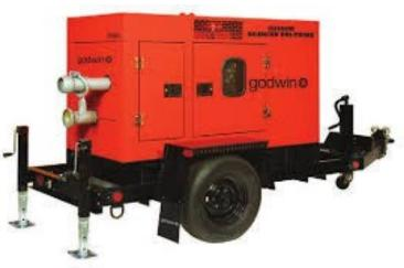
These pumps pump the flow through large black pipes and then dump the flows in a downstream manhole.
