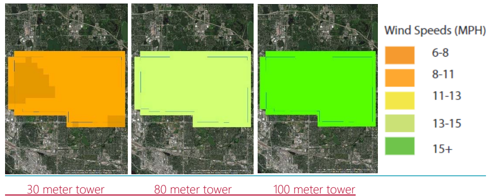
Figure X Wind speeds at different tower heights in Roseville, 30 meters, 80 meters, and 100 meters from left to right. Source: MN Department of Commerce
