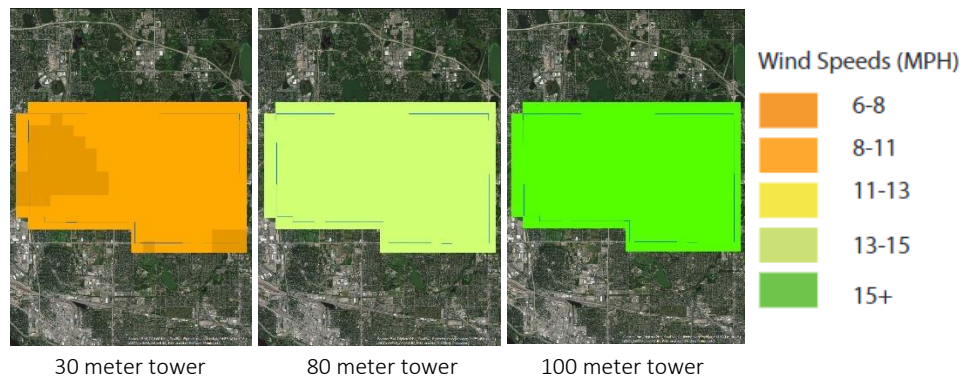
FIGURE 9-4 WIND SPEEDS AT DIFFERENT TOWER HEIGHTS IN ROSEVILLE. SOURCE: MN DEPARTMENT OF COMMERCE.
