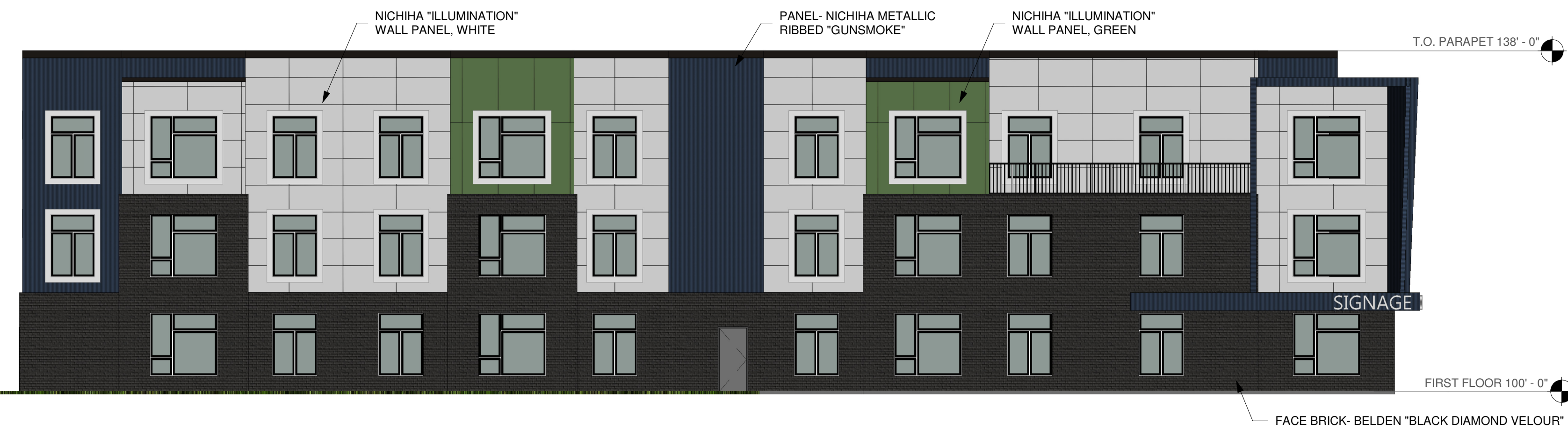
3 S OWASSO BLVD ELEVATION A401 1" = 10'-0"
