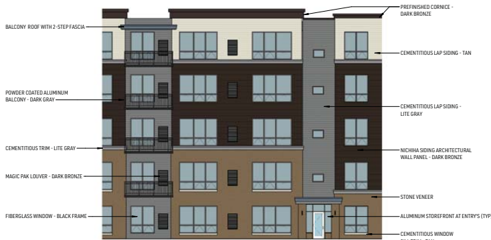
ELEVATION DIAGRAM 3/32" = 1'-0"
