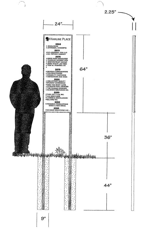
2" SQUARE ALUMINUM TUBE FRAME WITH 1"--"F" RETAINER. NON-GLARE ACRYLIC VANDAL COVER STEEL BACK PLATE WITH WHITE MAGNETIC TENANT STRIPS. BLACK REFLECTIVE VINYL TENANT COPY .85" TALL.
