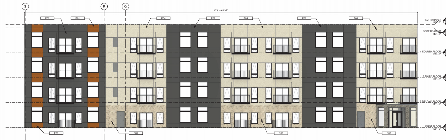
2 A404 EXTERIOR ELEVATION NORTH - SOUTH WING Copy 1 1/8" = 1'-0"
